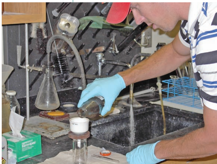
Simazine was extracted (shaken) from soil for four hours using methanol.
